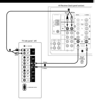
Figure 8. Connecting the A/V Receiver.
